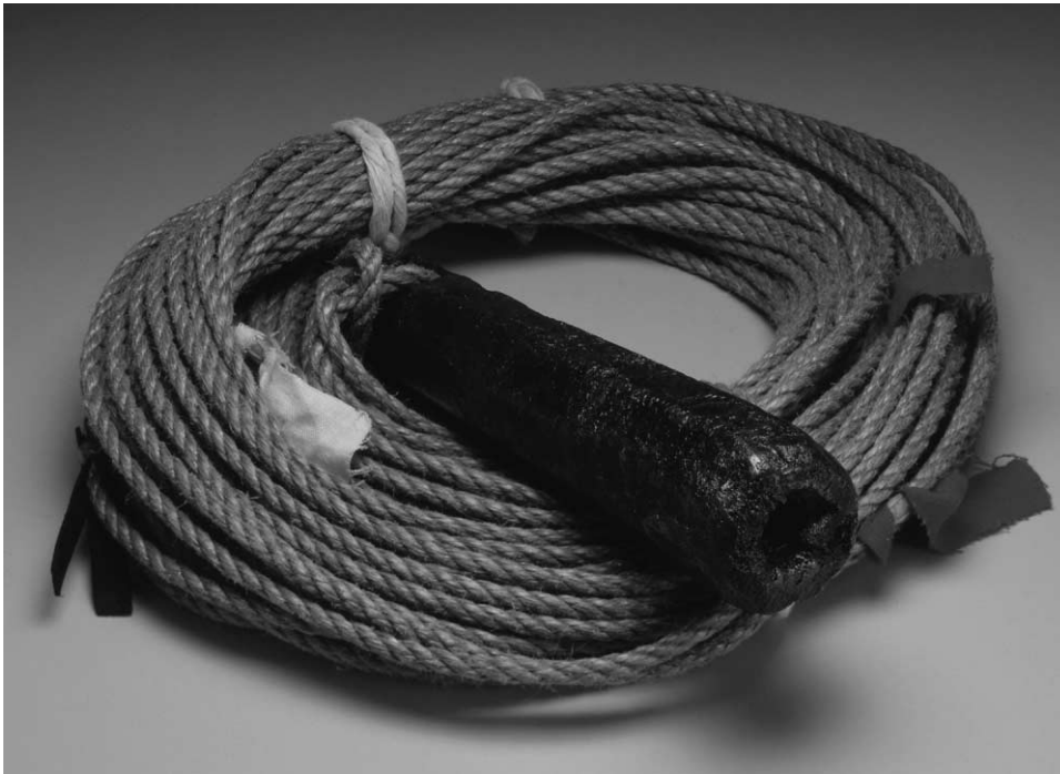
Figure 2. A sounding lead (pronounced like the metal from which it is made) and line. This hydrographic tool became crucial to Darwin’s work as a naturalist. A “hand lead” such as this one would have been roughly 8–12 inches tall and 6–12 pounds in weight. The base of the lead features a depression known as a “well,” which would be “armed” with soft tallow or wax. By this method a sample from the seafloor (or an impression of the bottom if it were clean) could be recovered. During the Beagle voyage Darwin made innovative use of his shipmates’ soundings as a method for acquiring geological, zoological, and botanical specimens from the seafloor. The epistemic value of these specimens was enhanced by the fact that geographical data (about the depth and location at which they had been found) was appended to them as an intrinsic feature of the surveyors’ work. (Image: The Mariner’s Museum.)
